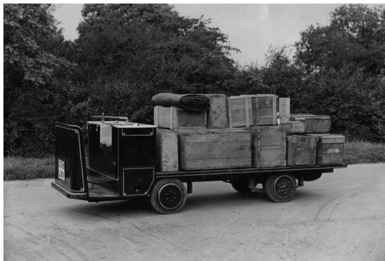
*The very original S.D. Freighter, though in appearance possessing much in common with the works truck, is designed for road work at speeds up to 14 m.p.h., and its careful springing and weight distribution afford exceptionally easy riding, even over 'pot holey' roads*
